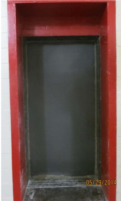
Figure 1 - Specimen mounted in the test opening.
