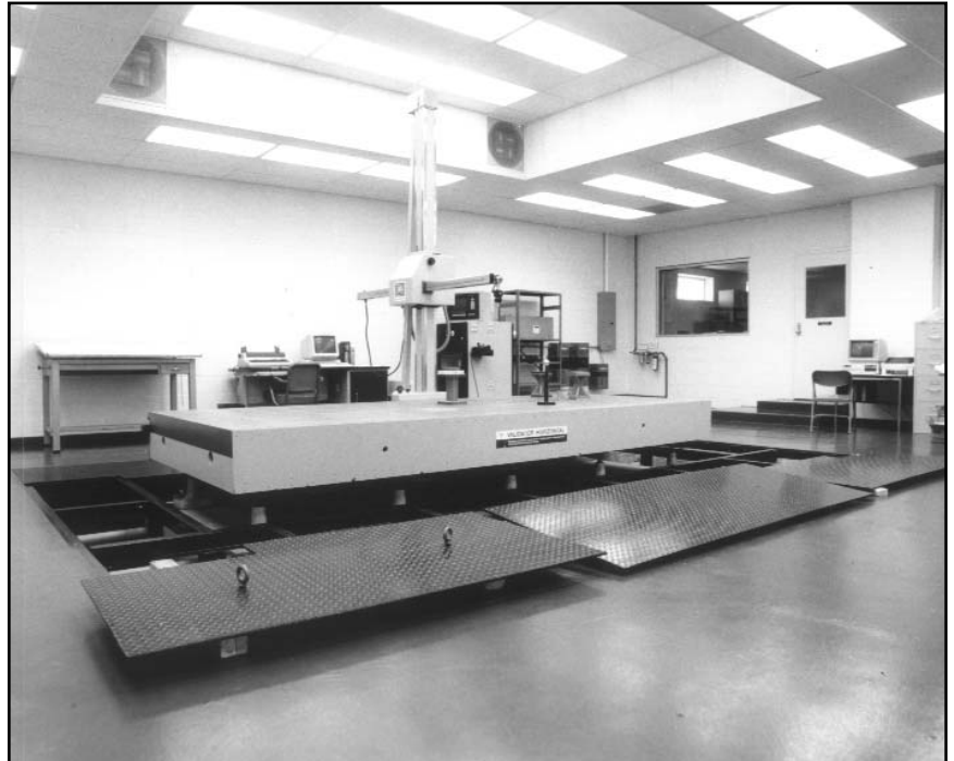
Single Arm CMM on Air Support Inertia Base with Removable Isolator Access Plates
