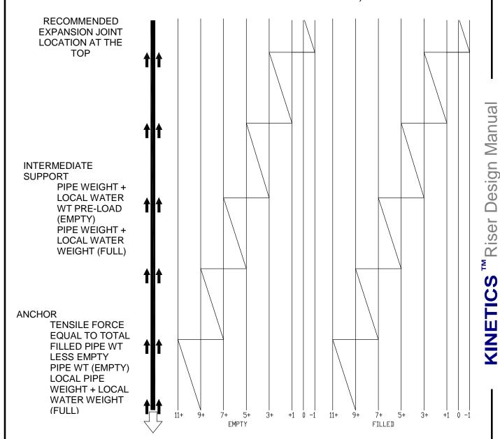
RELATIVE PIPE STRESS ASSUMING PIPE WT/FT AND WATER WT/FT IS APPROXIMATELY EQUAL (12' STD WT PIPE)
