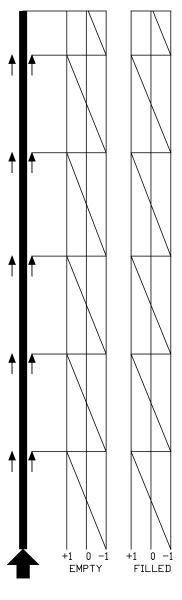
RELATIVE PIPE STRESS ASSUMING PIPE WT/FT AND WATER WT/FT IS APPROXIMATELY EQUAL (12" STD WT PIPE)
