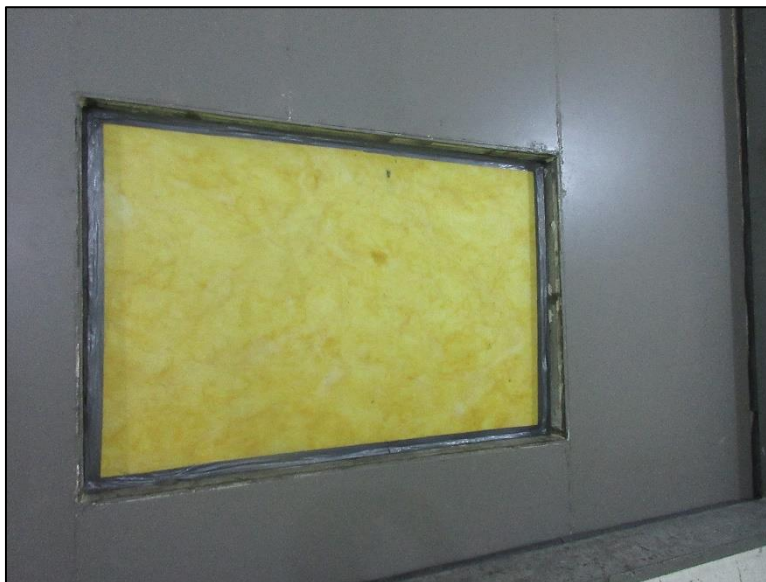
Photo No. 2 Source Room View of Installed Test Specimen
