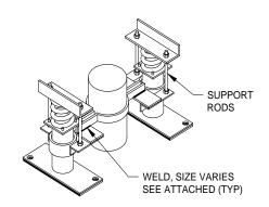
can be offset to allow the full range of growth/shrinkage to be accommodated over the active travel range of the guide. The riser clamps can now be securely tightened against the pipe and welded to the sliding element. When welding the riser clamp or bracket, the weld should be done in a series of small passes allowing adequate time in between for cooling to protect the internal rubber elements in the sliding element itself.
