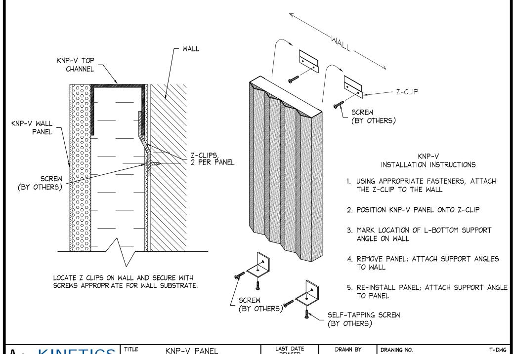
KNP-V PANEL INSTALLATION WITH Z-CLIPS AND L-BOTTOM SUPPORT ANGLES
