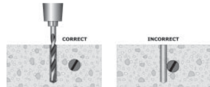
Figure 130: Drilling into concrete with rebar.
