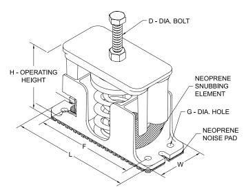
or as indicated on the project documents. Springs shall be color coded or otherwise identified to indicate load capacity.
