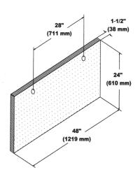
Larger baffles up to 48" x 96" available with 2" thick fiberglass core
