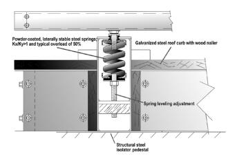
The upper support rail shall consist of a structural channel with sufficient elevation above the spring to preclude interference with the rooftop equipment and permit access to inspect the isolation system after placement of the rooftop equipment. Support of the RTU by weather seal attachment bolt heads is not permitted.
