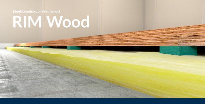
RIM is an easy to install, high-performance noise control system. The rolls of RIM use acoustic batting to prespace isolation pads which forms an airspace—an essential component for noise control.
