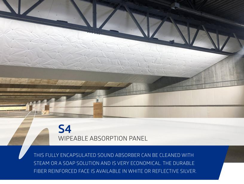
**S4 Panel** is an economical and easily cleanable sound absorber. The S4 panel is constructed from a 3 PCF fiberglass core completely encapsulated with a fiberglass reinforced, aluminized polyester film facing. S4 is available in 1" and 2" thicknesses and panel sizes up to 48" x 120". The S4 panel with aluminized (silver) facing can be used in temperatures from -65° F to 265° F.
