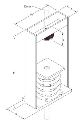
Isolation hangers shall be selected by the manufacturer for each specific application to comply with deflection requirements as shown on the Vibration Isolation Schedule or as indicated on the project documents.
