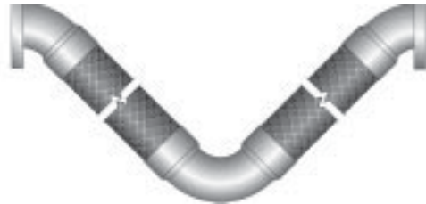
Figure 137: Braided hose expansion joint.
