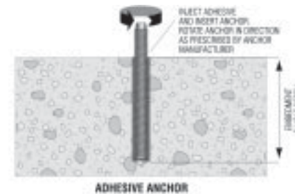
Figure 110: Adhesive anchor installation.
