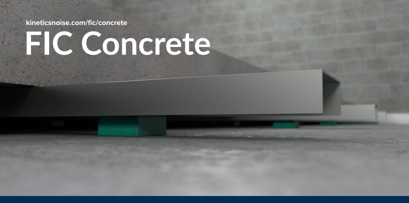
An acoustic airspace is formed by adhering pre-spaced KIP isolation pads to steel channel. This isolated framing platform is a base for either metal decking as a formwork for concrete or to directly attach concrete structural panels.
