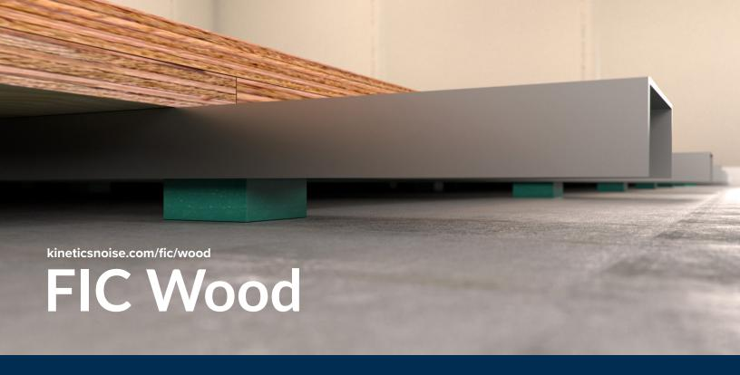
An acoustic airspace is formed by adhering pre-spaced KIP isolation pads to steel channel. This isolated framing platform is a base for lightweight noise control construction using a plywood composite.
