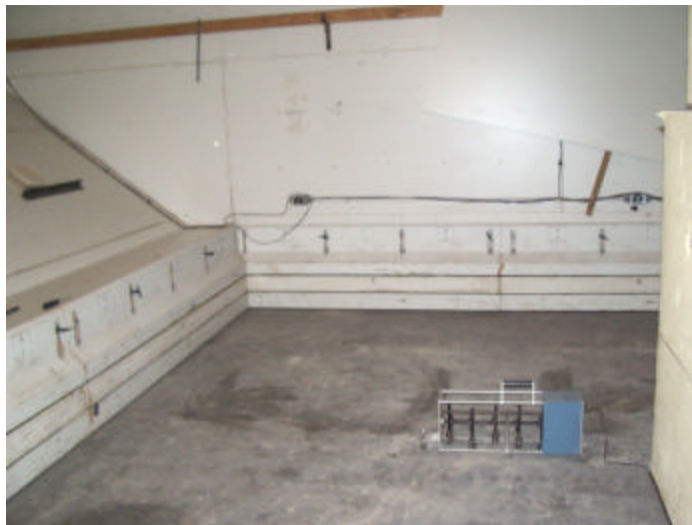
Figure 1: The NRC reference concrete slab installed in the floor test frame.
