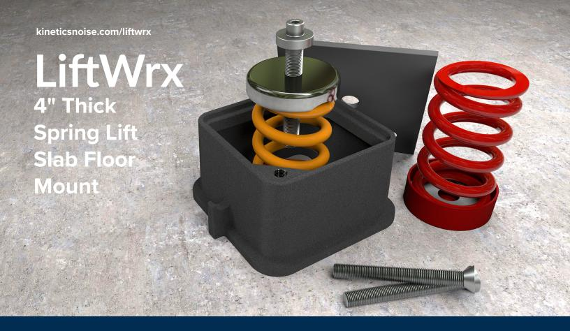
Lift slab floating floor systems that incorporate spring isolator assemblies to decouple four inch thick concrete slabs from non-isolated structural floors are used where vibration and impact are critical and of greater concern than airborne noise transmission.
