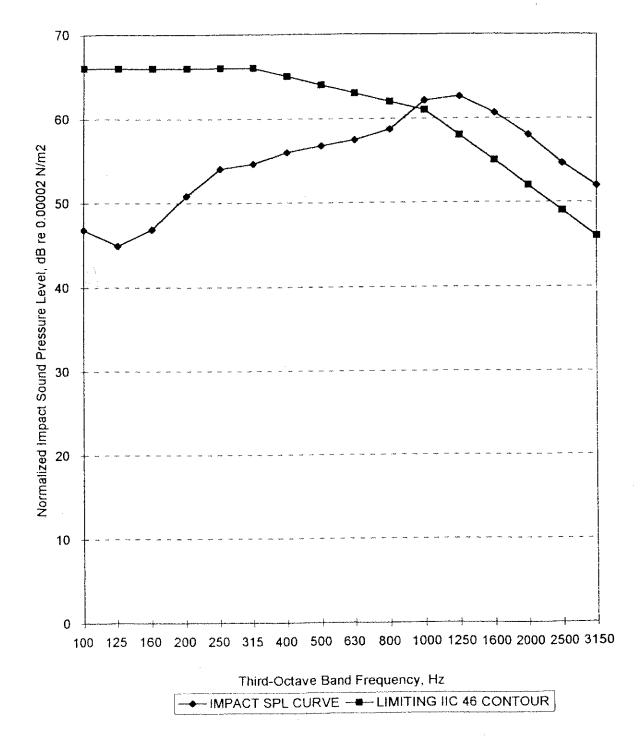
The IIC value was determined by applying the Averaged Sound Pressure Levels (SPL) values to the IIC reference contour of ASTM E1007-97, Field Measurement of Tapping Machine Impact Sound Transmission Through Floor-Ceiling Assemblies and Associated Support Structures.
