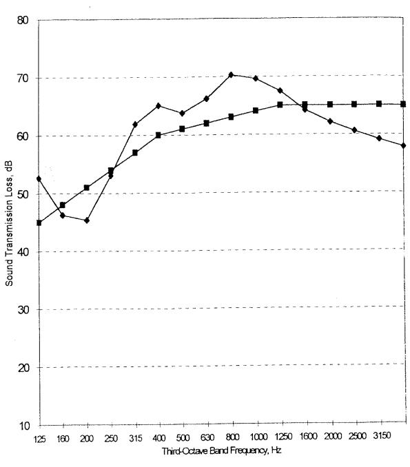
The STC value was determined by applying the Transmission Loss (TL) values to the STC reference contour of ASTM E413-87, <u>Determination of Sound Transmission Class.</u>
