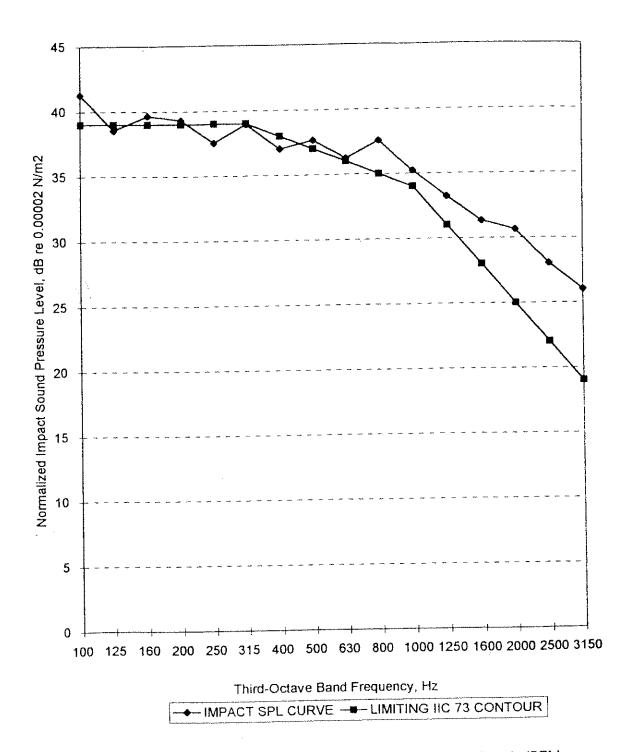
The IIC value was determined by applying the Averaged Sound Pressure Levels (SPL) values to the IIC reference contour of ASTM E1007-97, <u>Field Measurement of Tapping Machine Impact Sound Transmission Through Floor-Ceiling Assemblies and Associated Support Structures.</u>
