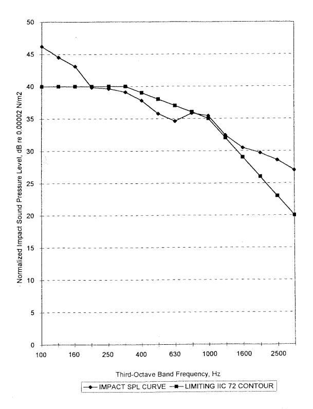
The IIC value was determined by applying the Averaged Sound Pressure Levels (SPL) values to the IIC reference contour of ASTM E1007-97, Field Measurement of Tapping
