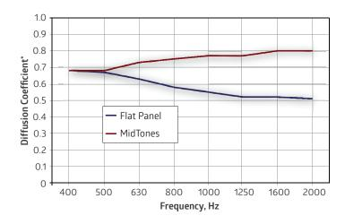
\*MidTones diffusion coefficients based on reduced scale model testing. Actual performance may vary.
