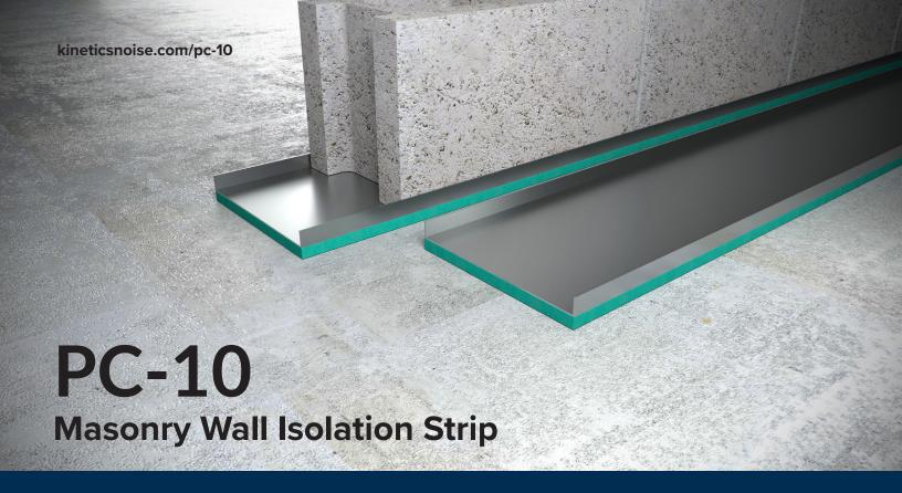
Kinetics Noise Control's PC-10 is a custom-molded and coated fiber glass board with galvanized steel channel which resiliently decouples a CMU (concrete masonry unit) wall from non-isolated structure.
