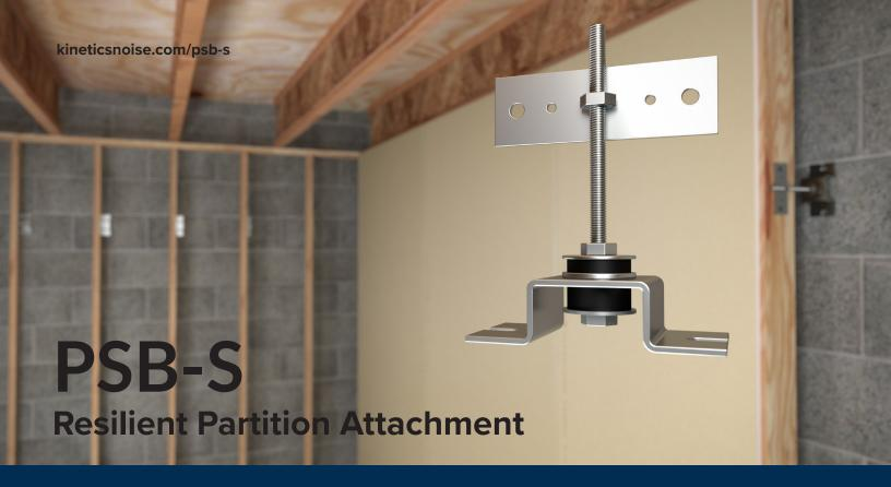
For use when wall isolation is desired for wood-and steel-frame studwall construction, PSB-S supports the partition from buckling and eliminates the "give" felt when leaning on a wall that is acoustically isolated. PSB-S can be implemented in many construction situations, as it is a multi-axis restraint and is seismically rated.
