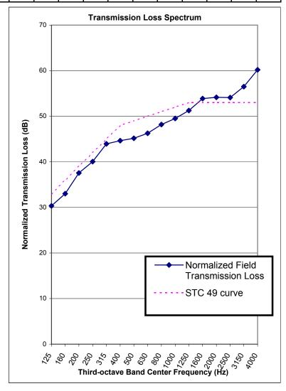
This test procedure was based on ASTM Standard E336.
