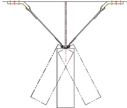
In order to keep this swaying motion from occurring, it is necessary to ensure that on the axis where swaying can occur, the restraints connect to the equipment at its vertical center of gravity (approx). This is not necessary on the opposite axis. See Below.
