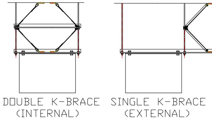
**Figure D10.6.3; Wall Penetration Restraint (Cable)**
