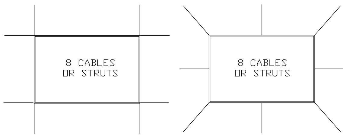
**Figure D10.4.2-3; 4 Strut Arrangement, Restraint angles can vary 10 degrees from those**
