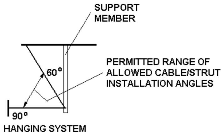
When installing restraints, each individual restraint should be installed perpendicular ( $\pm 10$  degrees) to the adjacent restraint as viewed from underneath. In addition, the restraints should be approximately aligned with the center of gravity of the piece of equipment being restrained. Although it is typical to install restraints at each corner extending radially outward from the piece of equipment, this arrangement is not mandatory. See the sketches below.
