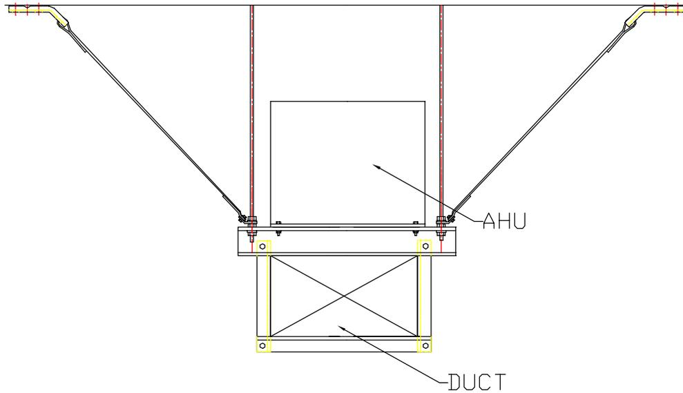
It is possible under some conditions to brace one trapeze bar to the other, and then restrain the second trapeze bar to the structure. This is shown below:
