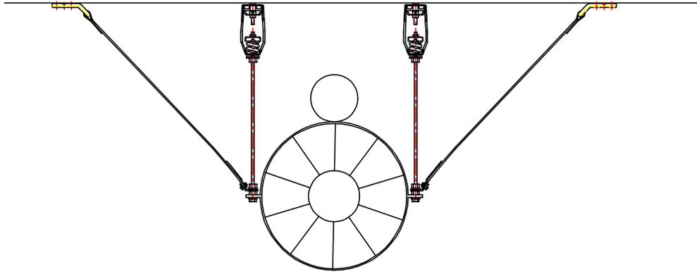
Most equipment however is mounted using a trapeze bar arrangement. There are many options that exist for the arrangements of restraints used in conjunction with trapeze-mounted systems. Shown below are several options for both non-isolated and isolated cable-restrained systems.
