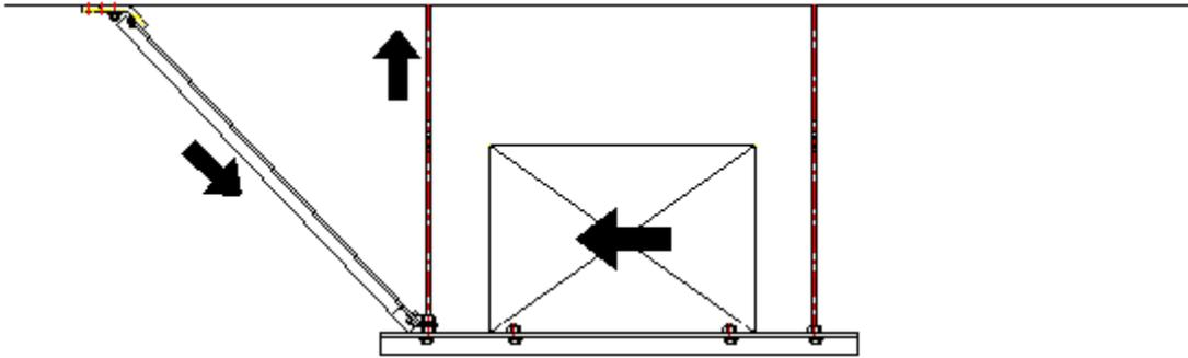
The key factor to note is that cables can only be loaded in tension. This means that seismic forces can only generate compressive loads in the hanger rod. Seismic forces can, however, load the strut in compression resulting in a tensile load on the hanger rod.
