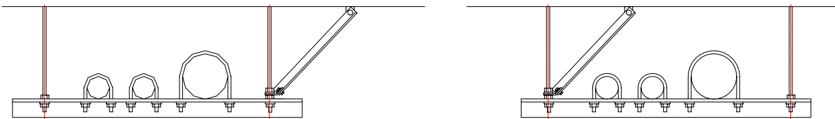
Figure D9.4.2-8; Shown below are 3 options for trapeze-supported conduit. All are equivalent.
