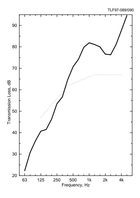
Figure 1: Airborne sound transmission loss measurements of Floor "C". The solid line is the experimental data, the dotted line is the STC 63.
