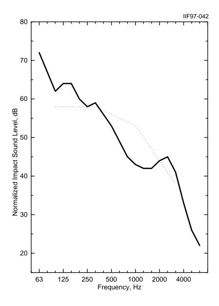
Figure 2: Impact sound transmission measurements of Floor "C". The solid line is the experimental data and the dotted line is the IIC 54 contour.
