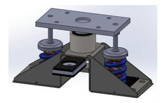
Slide the Vertical Restraint Component out of the Housing
