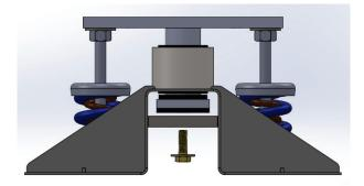
Unscrew and remove the Vertical Restraint Bolt
