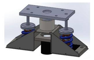
The Horizontal Restraint Element will Drop out of the Housing
